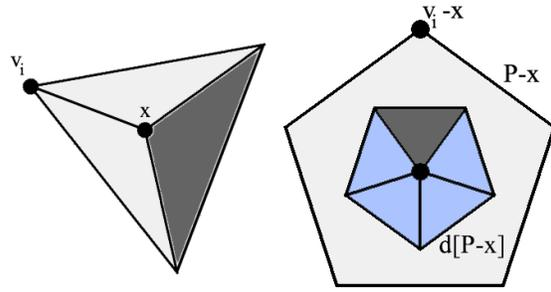
**Figure 3:** The simplicial formula for  $b_i$  is the ratio of the shaded area to the area of the triangle (left), but does not extend beyond simplices. Barycentric coordinates for a pentagon via partitioning of its dual (right). The coordinate  $b_i$  for  $v_i$  is the ratio of the dark area to the entire shaded dual.
