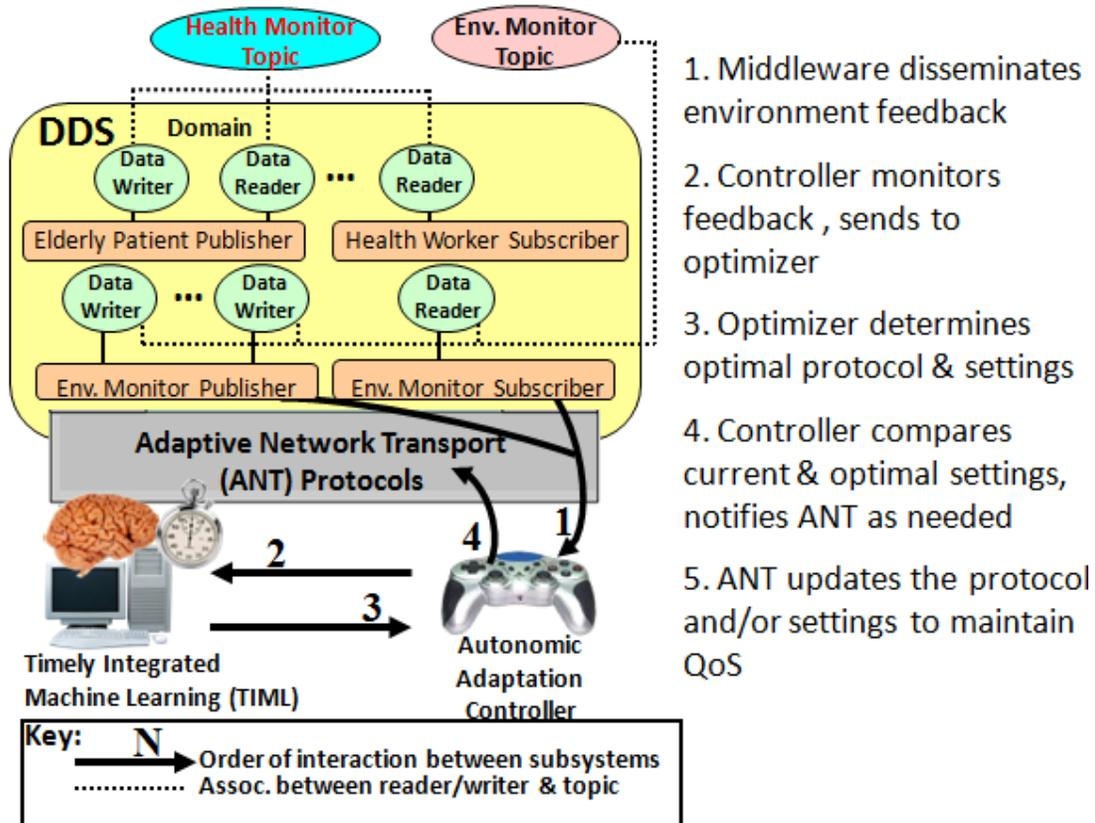
Figure 2: ADAMANT Architecture and Control Flow
