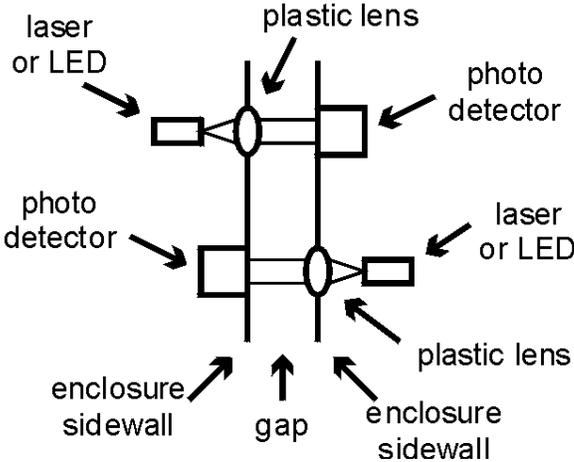
Figure 7: Topology for Bi-directional Link
