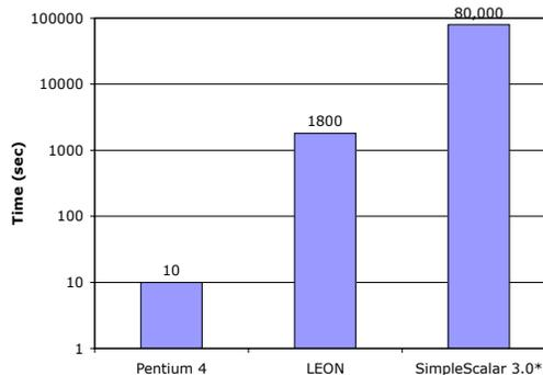
Figure 6: Time to run our application on a Pentium, on our reconfigurable platform, and on a (software) simulator to obtain cache-usage statistics.
