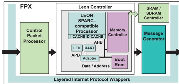
Figure 1: High-level architecture of the Liquid processor system
