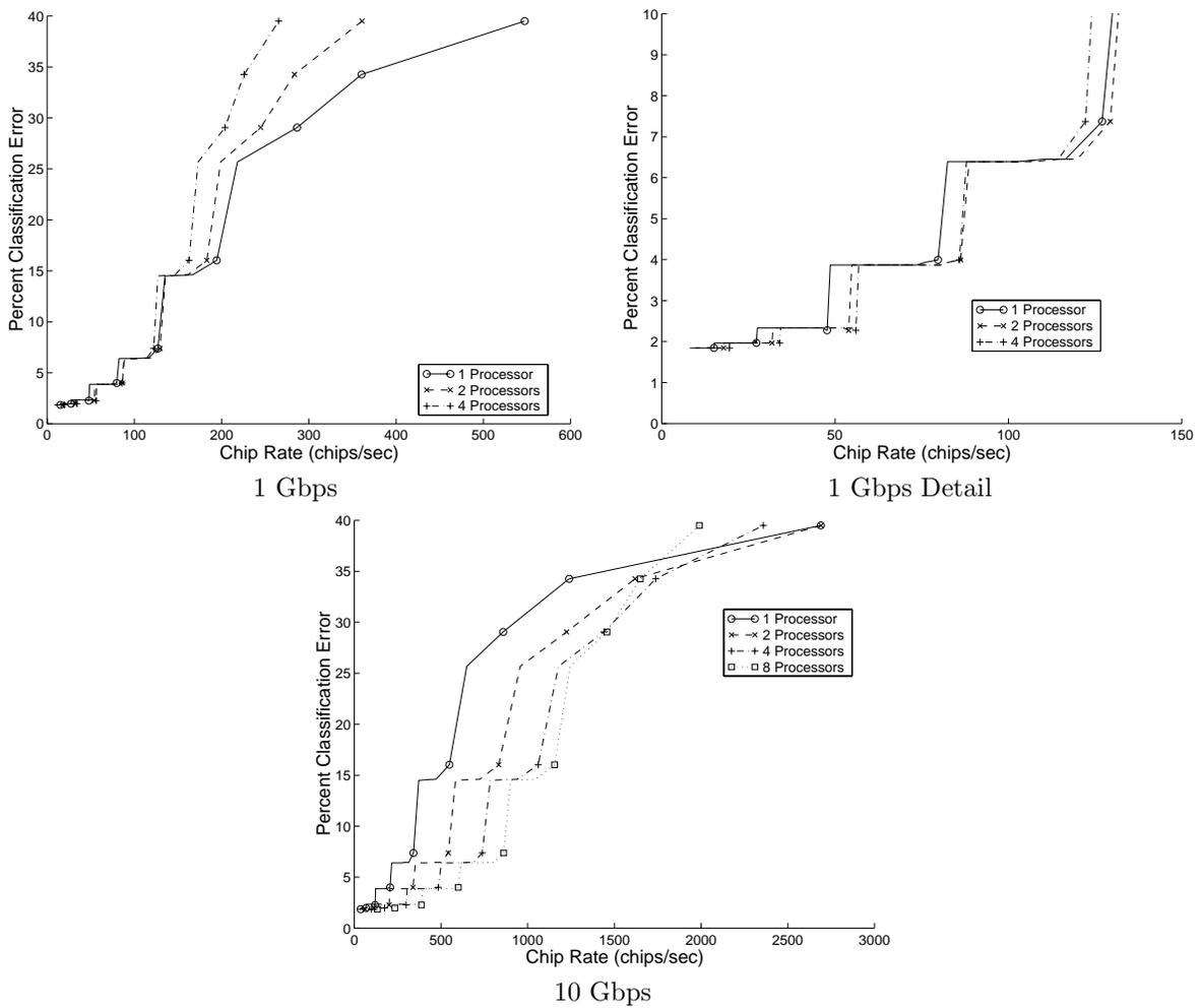
**Figure 3.** Percent classification errors as a function of chip throughput in a four-class experiment. Left panel shows results with 1 Gbps interconnection network. Right panel shows detail view of transition region with 1 Gbps interconnection. Bottom panel shows the much higher throughput attainable with a 10 Gbps interconnection.
