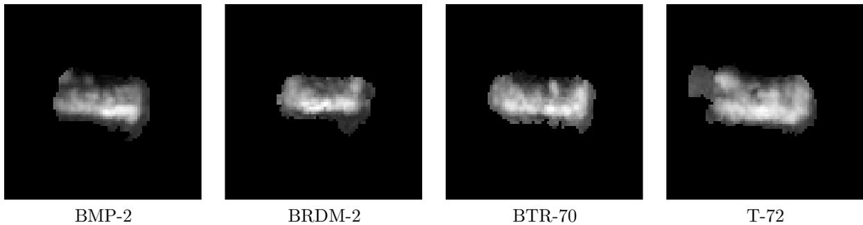
**Figure 2.** Masked models of sensor output for each of the four targets oriented  $90^\circ$  relative to the SAR platform with variance functions approximated as piecewise constant over 32 intervals.
