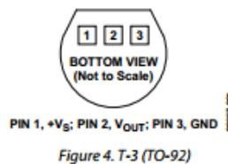
You should connect pin 1 to +5V, pin 2 to an analog input pin, and pin 3 to GND.
