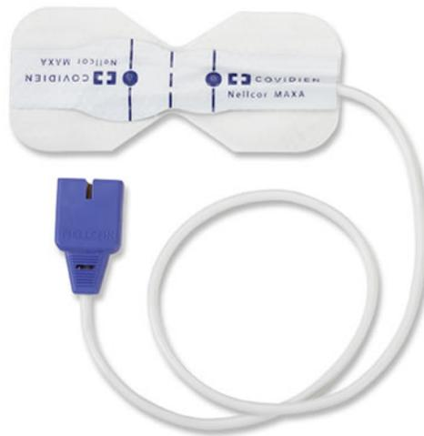
The probe houses a light source (both a red LED and an infrared LED, we will only use the red LED) and a light detector (photodiode). The probe is placed on the finger so there is a light-transmitting path from the source to the detector through a finger. As the blood flow pulsates in the arteries, the amount of light detected varies, and the signal from the light detector is used to measure pulse.
