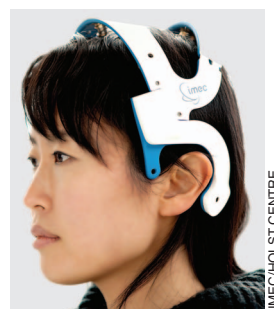
A prototype headset, developed at the IMEC/Holst Centre, is capable of recording high-quality EEG signals and transmitting them wirelessly in real time to a receiver at distance up to 10 m away.
