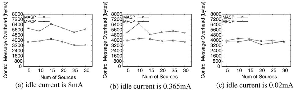
Fig. 16. Routing overhead on different platforms.
