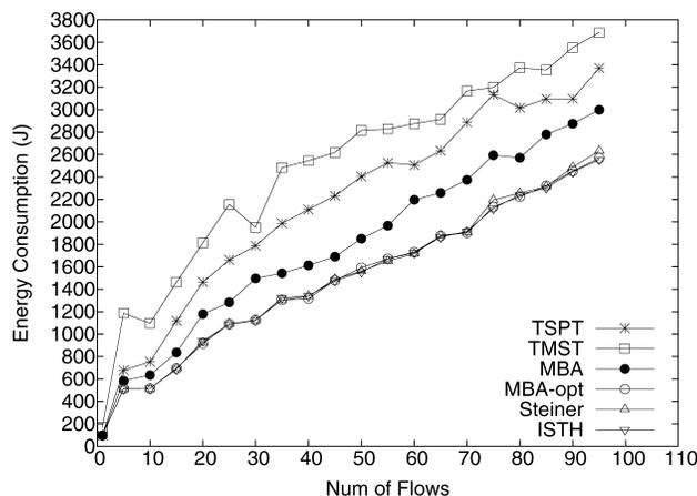
Fig. 9. Energy consumption vs. number of flows. The data rate of each flow is 0.2Kbps.
