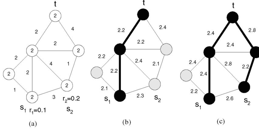
Fig. 5. (a) Initial network with edge weight  $C_{u,v}$  and node weight  $z = 2$  (shown on each node). (b) edge weights are defined by  $r_1 \cdot C_{u,v} + z$ . (c) edge weights are defined by  $r_2 \cdot C_{u,v} + z$ . The shortest paths from  $s_1, s_2$  to  $t$  are highlighted in black.
