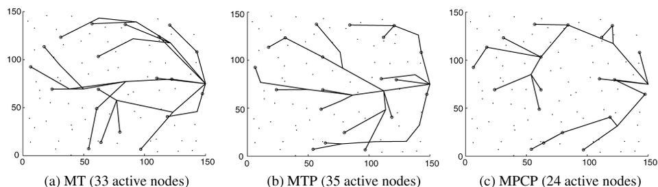
Fig. 11. Routing topologies of different protocols with 20 sources.
