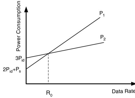
Fig. 2. Average power consumption vs. data rate.
