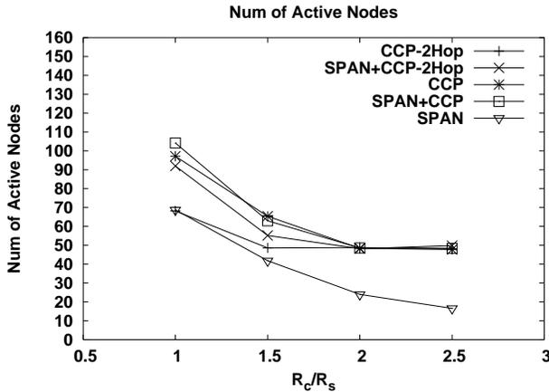
Figure 16. Number of Active Nodes vs.  $R_c/R_s$
