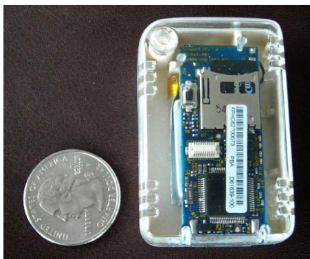
Fig. 1. The SHIMMER wearable sensor platform. SHIMMER incorporates a TI MSP430 processor, a CC2420 IEEE 802.15.4 radio, a triaxial accelerometer, and a rechargeable Li-polymer battery. The platform also includes a MicroSD slot supporting up to 2 GB of Flash memory.
