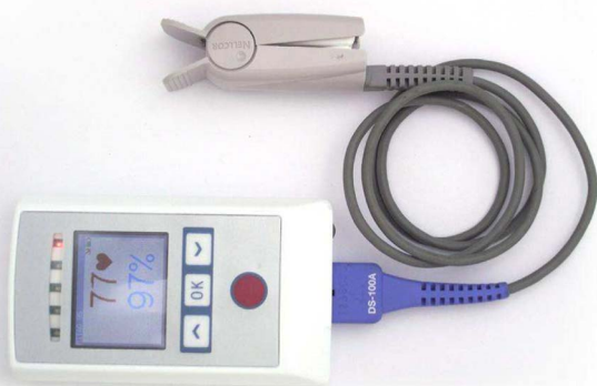
Fig. 2. Medical information tag, or miTag for short, used in MEDiSN [43]. The miTag is a Tmote mini-based [53] patient monitor that includes a pulse oximetry sensor with LEDs, buttons and an LCD screen. The miTag is powered using a rechargeable 1200-mAh 3.7-V Li-Ion battery and external finger tip sensors are used to make the pulse oximetry measurements.
