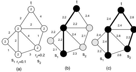
Figure 5: (a) Initial network with edge weight  $C_{u,v}$  and node weight  $z = 2$  (shown on each node). (b) edge weights are defined by  $r_1 \cdot C_{u,v} + z$ . (c) edge weights are defined by  $r_2 \cdot C_{u,v} + z$ . The shortest paths from  $s_1, s_2$  to  $t$  are highlighted in black.
