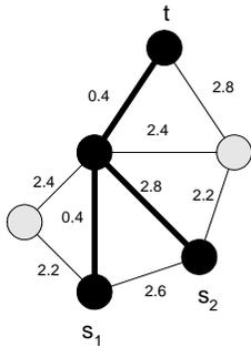
**Figure 7: The shortest path from  $s_2$  to  $t$  shares an edge with the existing shortest path from  $s_1$  to  $t$ .**
