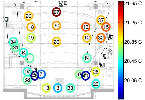
**Fig. 2: Measured temperature by wireless sensors and thermostats on Fri. Mar. 22, 2013 at 12 : 30pm, when the auditorium was fully occupied due to a seminar and HVAC was active (the background is the floor plan of the auditorium). Circles and numbers indicate locations and IDs of sensors respectively. The color bar (right) indicates corresponding temperature of each sensor. Sensor 40 and 41 represent thermostats.**
