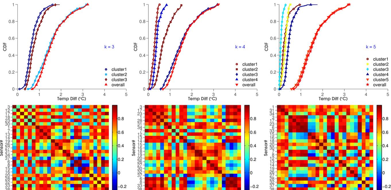
Fig. 7: Euclidean distance based clustering algorithms.  $k$  represents cluster number. The top row is distribution of maximum temperature differences while the bottom row is the correlation map.  $k = 3$  is chosen by the largest eigengap. Overall indicates the maximum temperature difference between all sensors in the auditorium
