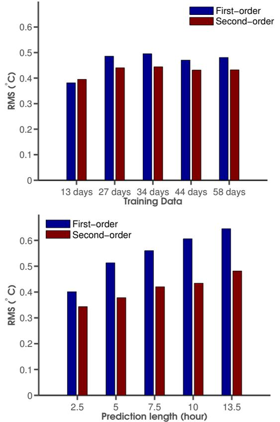
**Fig. 5: Temperature prediction error (in 90<sup>th</sup> percentile) as training data increases (top subfigure) and prediction length increases (bottom subfigure).**
