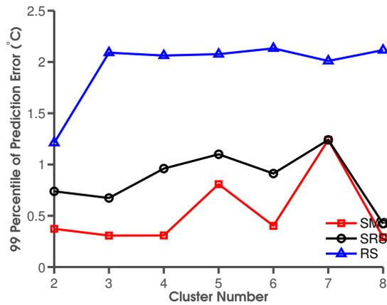
**Fig. 11: Comparison of accuracy of simplified model according to different sensor selection methods.**
