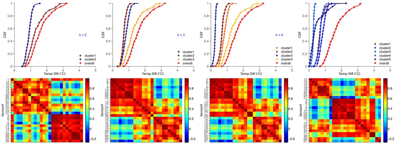
**Fig. 8: Correlation based clustering algorithms.**  $k$  is cluster number. The top row is distribution of maximum temperature differences while the bottom row is the correlation map.  $k = 2$  is chosen by *the largest eigengap*. Data labelled as *Overall* indicates the maximum temperature difference between all sensors in the auditorium
