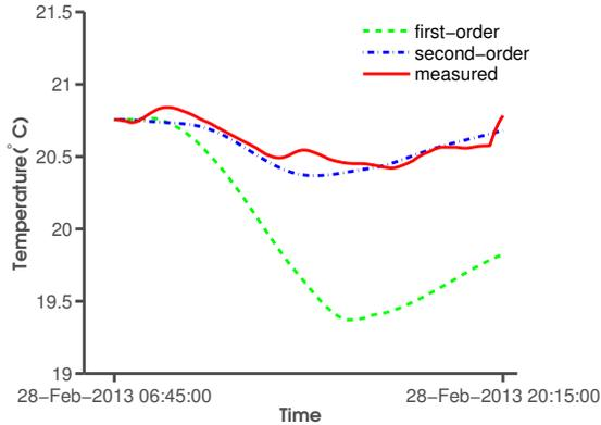
**Fig. 4: Temperature of the auditorium measured by sensor 1 and temperature estimated by first-order and second-order model in March 25, 2013.**
