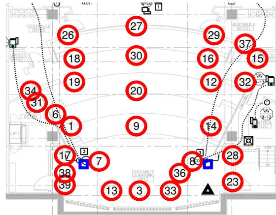
**Fig. 1: The auditorium and sensors. Red circles represent temperature and humidity sensors. Blue squares are the existing thermostats of the HVAC system while the black triangle is a web camera.**
