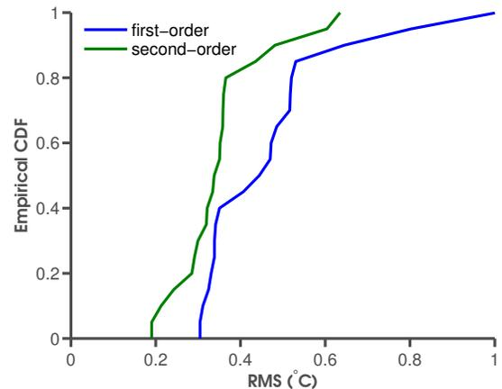
**Fig. 3: RMS of prediction error for all sensors in first-order and second model under occupied mode (Prediction window length is 13.5 hours for each day).**
