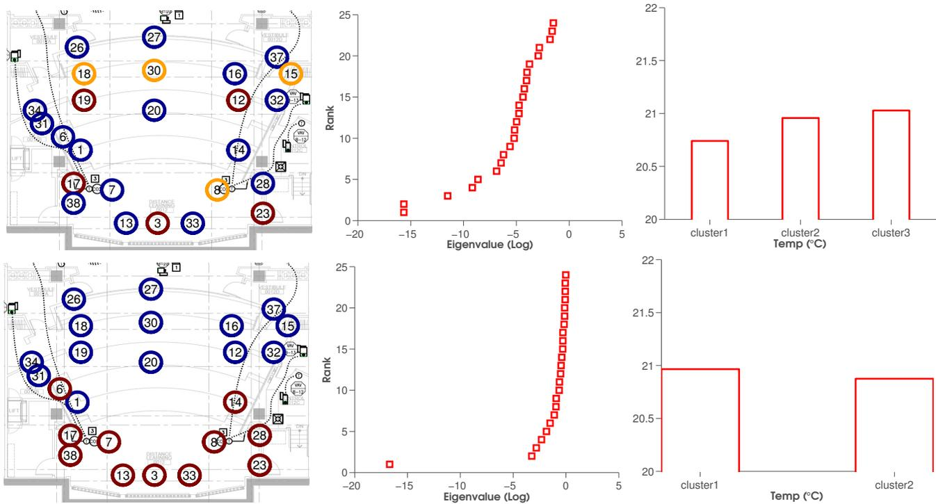
Fig. 6: Clustering sensors based on Euclidean distance (top) and correlation (bottom). The left column indicates the locations of sensors while colors represent clusters. The middle column represents eigenvalues of Laplacian. The right column shows the mean temperature for each cluster.
