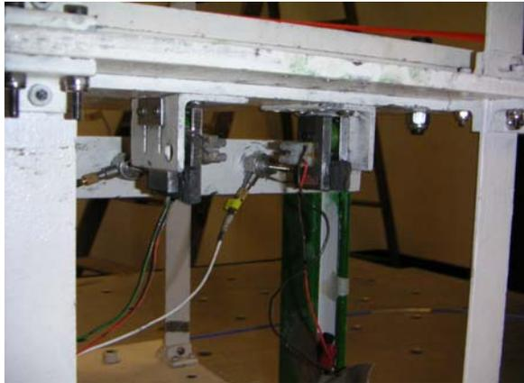
Figure 2 MR Damper Installation.
