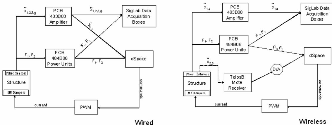
Figure 3 Schematic of the Wired (a) and Wireless (b) Experiments
