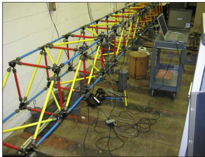
Fig. 9. 3D truss test structure
