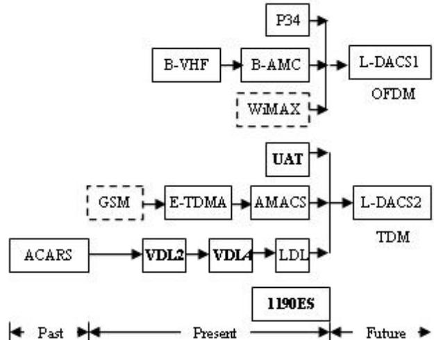
Fig. 1. Evolution of aeronautical datalinks
