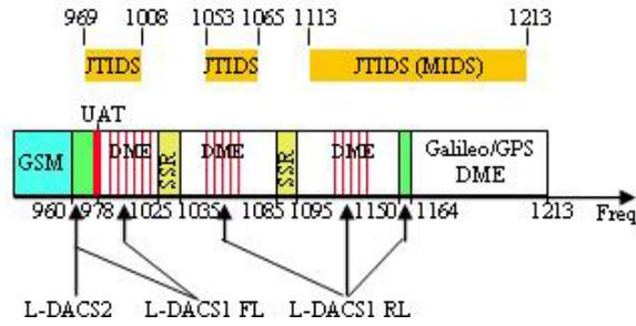
Fig. 4. L-band spectrum usage
