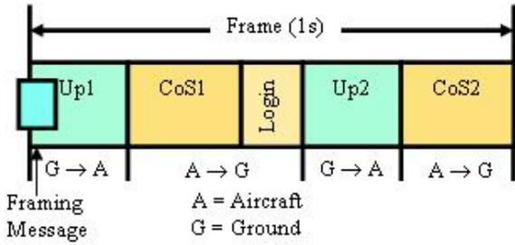
Fig. 3. L-DACS2 Physical Layer Framing
