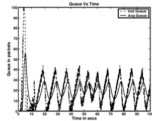
Figure 5. Queue for an unstable GEO Satellite Network
