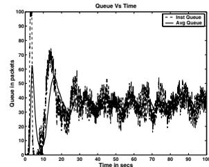
Figure 6. Queue for a stable GEO Satellite Network
