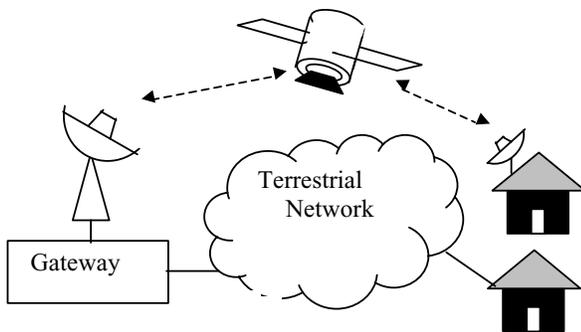
Fig. 1. Bent-pipe architecture.
