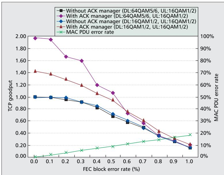
■ Figure 8. TCP goodput vs. block error rate.
