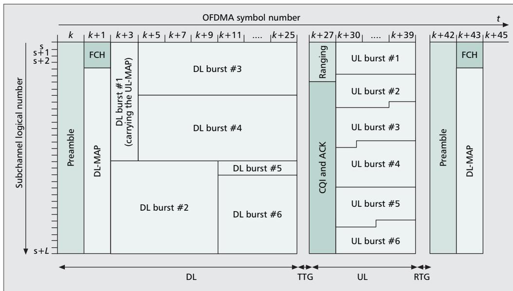
■ **Figure 1.** A sample OFDMA TDD frame structure.
