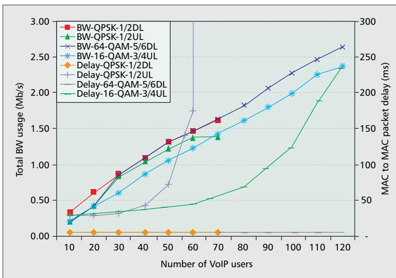
■ **Figure 5.** Number of VoIP Users: BW usage and packet delay perspective. DL/UL: (QPSK 1/2, QPSK1/2) and DL/UL: (64-QAM-5/6, 16-QAM-3/4).
