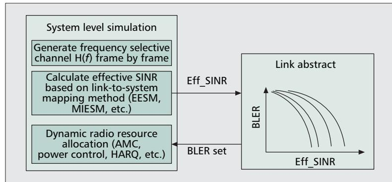
■ **Figure 6.** System-level simulation procedure and effective SINR mapping.
