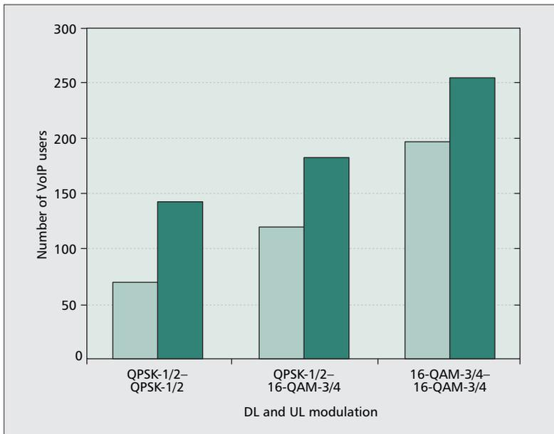
■ **Figure 4.** Number of VoIP users: BW usage perspective (without and with header compression).
