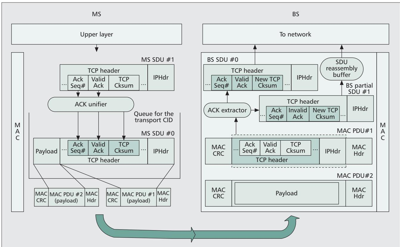
■ Figure 7. ACK manager: ACK unifier and ACK extractor.
