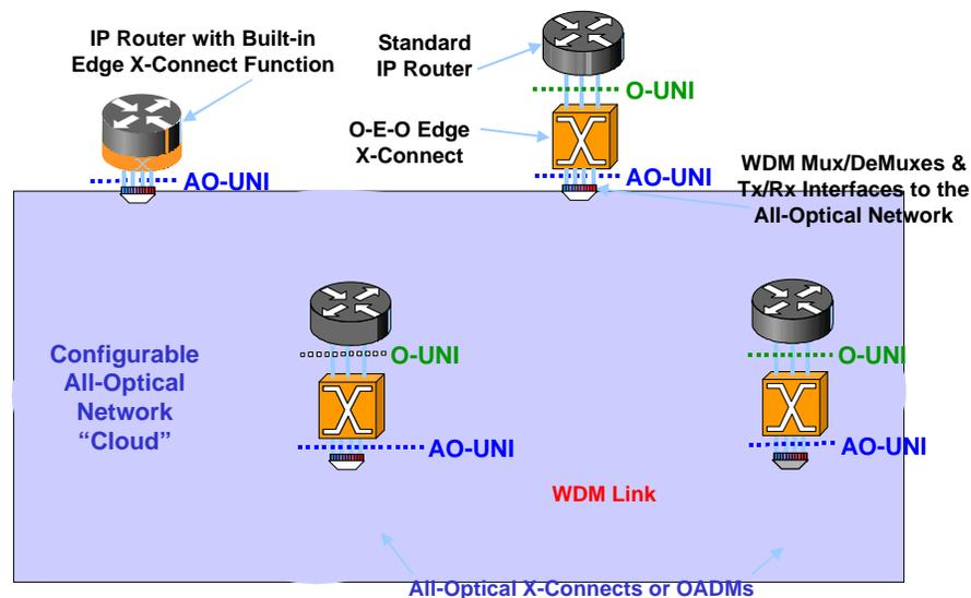
**Figure 1. REFERENCE MODEL 1:** *The Optical-User Network Interface (O-UNI) operates between the IP Router layer and the O-E-O Crossconnect layer, whereas the All-Optical UNI (AO-UNI) operates between the O-E-O layer and the All-Optical cloud. While the O-UNI can support a peer-to-peer model or client-server model, the recommended mode in Contribution OIF2000.278 for the AO-UNI is client-server.*
