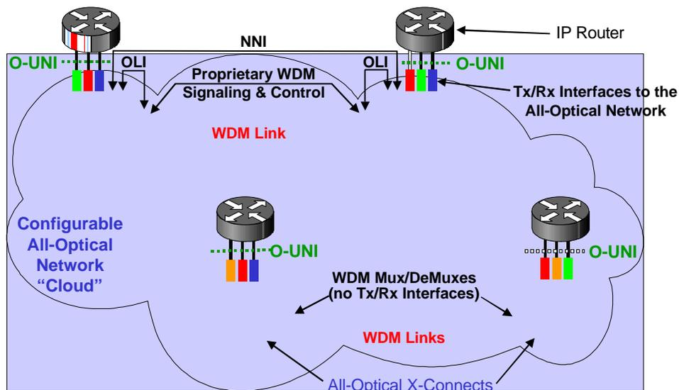
**Figure 2. REFERENCE MODEL 2:** In this model, which is proposed in Contribution OIF2000.254, emphasis is on signaling and routing within the all-optical network. An Optical Link Interface (OLI) is proposed to communicate performance monitoring information and WDM link system characteristics to the all-optical cross-connect layer. The use of such information to enable routing within the all-optical cloud was proposed in Contribution OIF2000.251.
