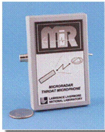
Fig. 8. Throat microphone using UWB radar( Image from LLNL MIR website, Livermore , USA ) [LLNL01]
