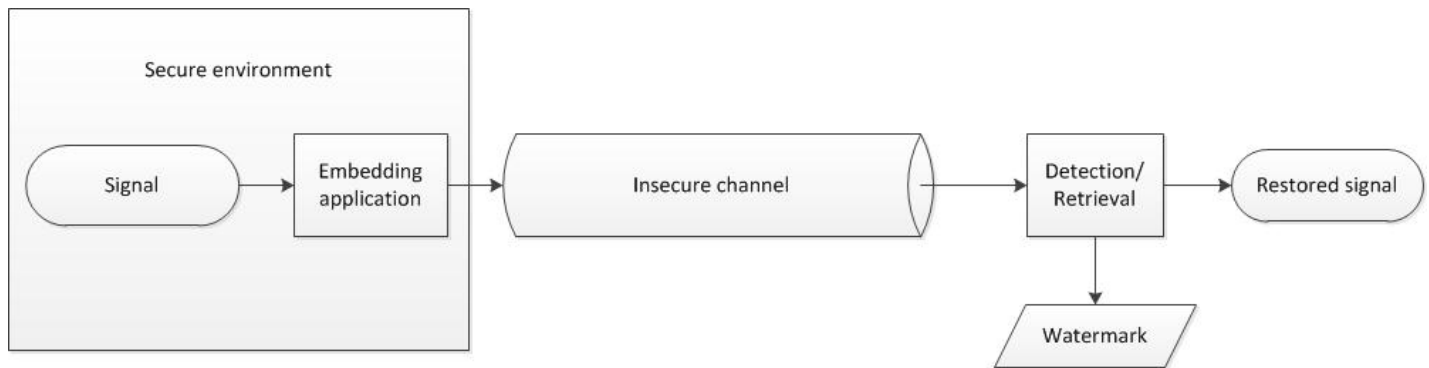
Figure 2. Life cycle of a digital watermark
