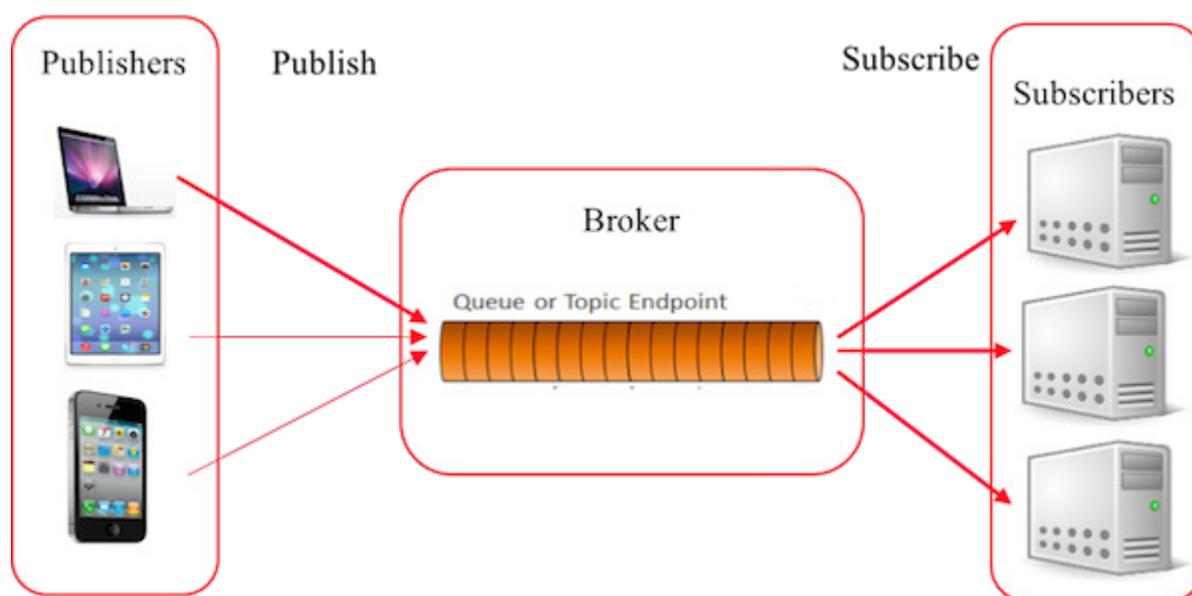
Figure 5: MQTT Architecture
