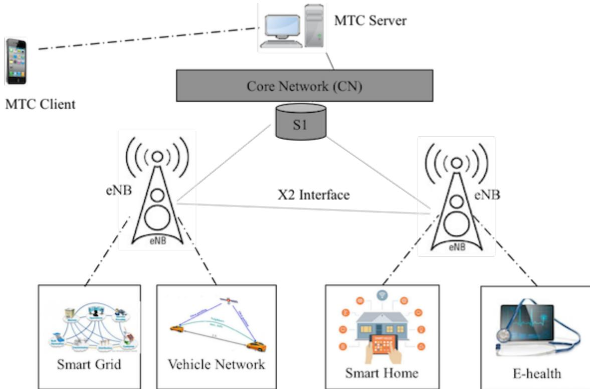
**Figure 4: LTE-A Architecture**
