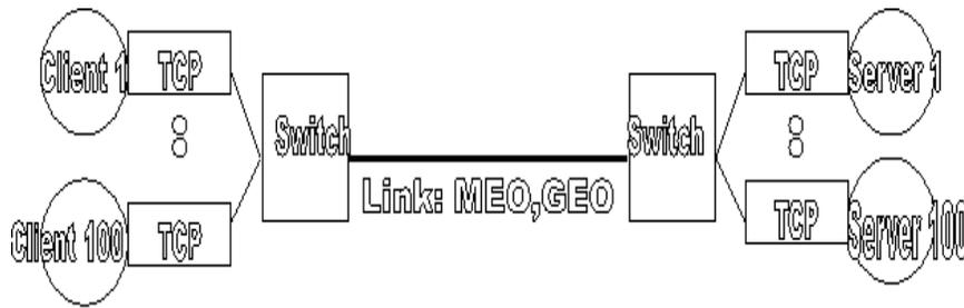
Figure 2 shows the configuration used in all simulations. The configuration consists of 100 WWW clients being served by 100 WWW servers, one server for each client. Both WWW clients and servers use underlying TCP connections for data transfer. The WWW traffic model used in this study is an extension of that specified in SPECweb96 benchmark. [11] and is based on HTTP/1.1 standard [1]. The switches implement the UBR+ service with optional drop policies described before.
