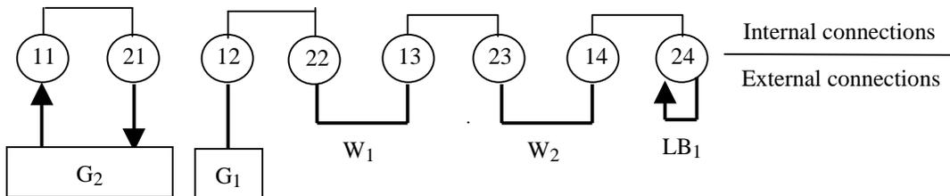
**Figure B.6.** The 6-to-6 straight configuration with one generator using inter-module VCCs, where the foreground traffic does not share any port with the background traffic.
