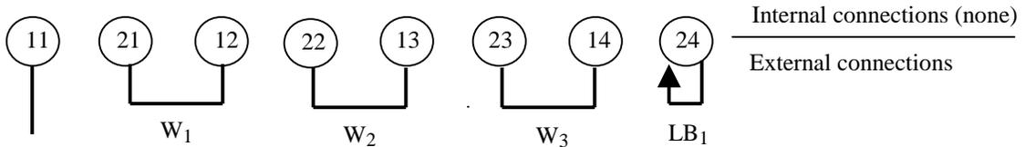
**Figure B.4.b.** Wiring configuration for the example switch.
