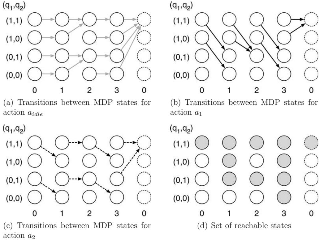
Figure 3.3: Wrapped utility-aware task scheduling MDP for a simple but illustrative example of two tasks with periods  $p_1 = 4$  and  $p_2 = 2$ , termination times equal to periods, and (deterministic) single quantum duration. Rows show states with the same valued indicator variables  $(q_1, q_2)$ , and columns show states with the same  $t_{system}$  value.
