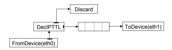
Configuration checking the TTL value of a packet
