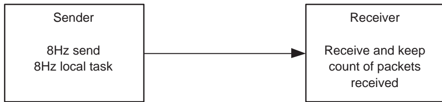
Figure 8: Experimental Setup for Packet Send Throughput
