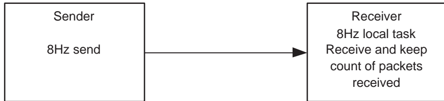
Figure 10: Experimental Setup for Packet Receive Throughput
