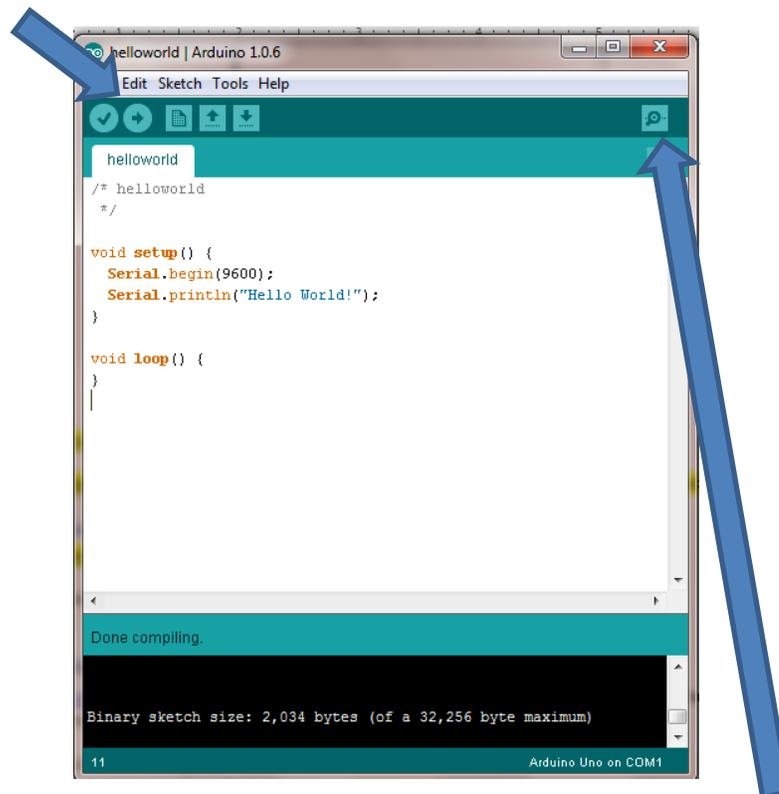
The window that displays the output can be opened using the Serial Monitor button. You might need to set which COM port via Tools -> Serial Port before this will work. Which COM port (e.g., COM3, COM4) will depend on which USB port you are using on the PC (it is unlikely to be COM1 or COM2).
