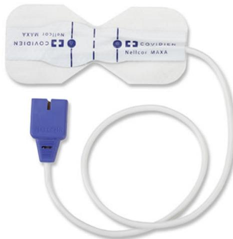
The probe houses a light source (both a red LED and an infrared LED, we will only use the red LED) and a light detector (photodiode). The probe is placed on the finger so there is a light-transmitting path from the source to the detector through a finger. As the blood flow pulsates in the arteries, the amount of light detected varies, and the signal from the light detector is used to measure pulse.
