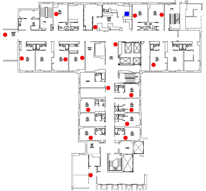
Figure 2. Deployment of the wireless clinical monitoring system in the step-down unit of Barnes-Jewish Hospital. The blue square denotes the base station. The red circles denote relay nodes.
