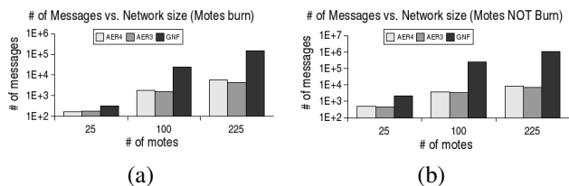
Fig. 3. Number of Messages. x-axis represents number of motes in the environment, logarithmic y-axis is number of messages. (a) When the motes fail in high temperature . (b) When the motes are not effect by fire.
